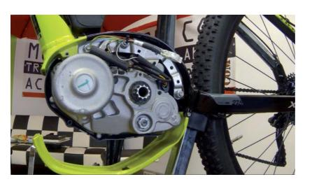
5. Pull the HMI 4-pin plug and the speed sensor 2-pin plug from the motor with flat nose pliers very carefully. Be aware to pull on the plug and not on the cables
