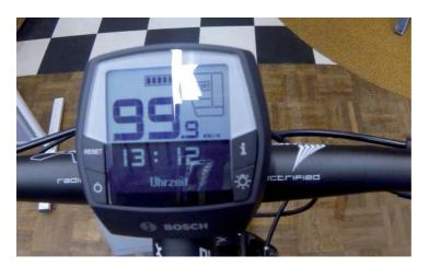
This is the calibration of the electronics, the electronics are determining the parameters in order to work correctly, depending on your e-bike. If the electronics show otherwise, check the connections.
