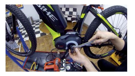
4. Remove motor cover by releasing the three Torx screws with a T20 screw driver.
