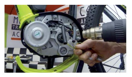
11. Place cables adequate, use cable binder to fasten the ASA eSPEED tuning module into the motor. Be careful, don't let the cables interfere with operating functions or be jammed in by the motor cover.
