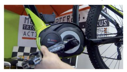
3. Remove crank with Cyclus crank extractor. The optional stone guard underneath the motor can now be removed with a 3 mm hexagon key
